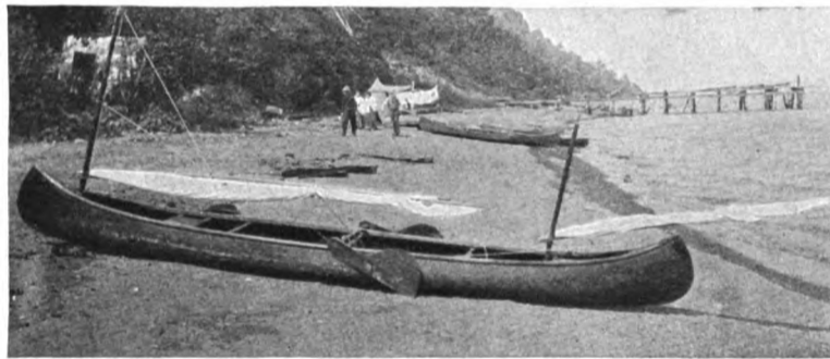
Open Canadian canoe fitted for sailing, with simple mainsail and mizzen, and folding leeboards, which can all be stowed in the canoe
