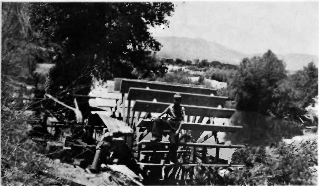
10-ft. Undershot Water Wheel - A. J. Ralston's place on Verde River - Pumps to small area formerly irrigated by C.V. Ditch. June 6, 1940.
