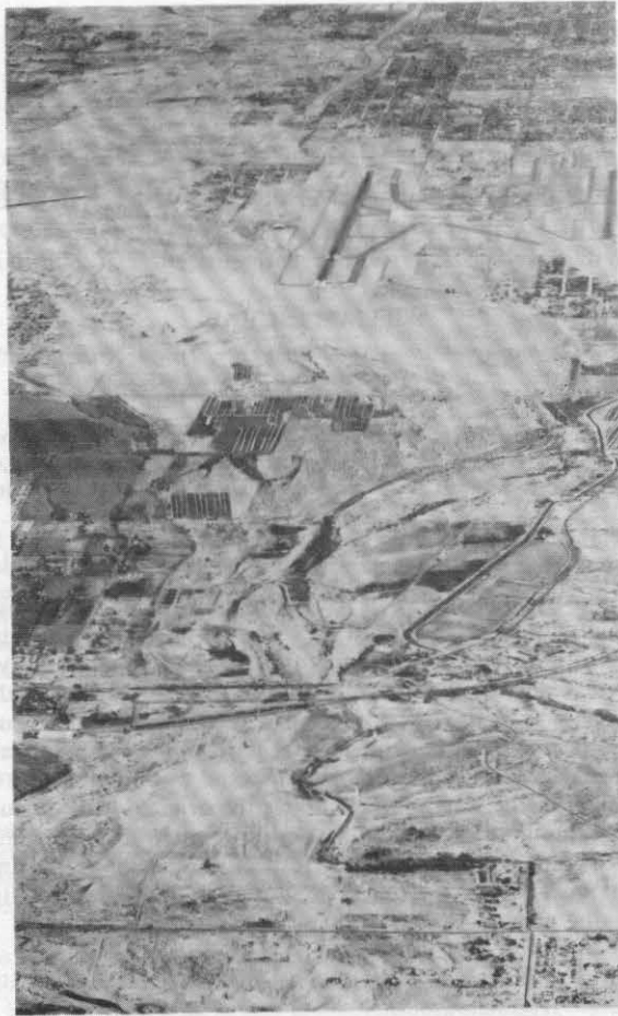
Figure 1. Channel of the Salt River near Tempe Butte looking west or downstream. A single main-flow or low-flow channel is outlined by vegetation in some areas. An artificially straightened reach occurs between the camera and the airport runway—it was destroyed and replaced by a slightly meandering channel in the flood of 1965. Photograph by Maddock Associates Aerial Surveys, held by the Phoenix Urban Study Office, U.S. Army Corps of Engineers (Frame 16, 15 September, 1962)
