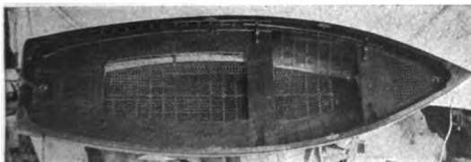
A 14-foot rowing boat arranged to be used as a yacht tender. Bronze trimmings
