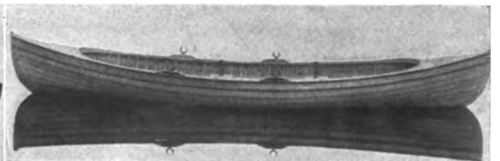
St. Lawrence skiff—a fine boat for rough water. Occasionally built to a length of 20 feet
