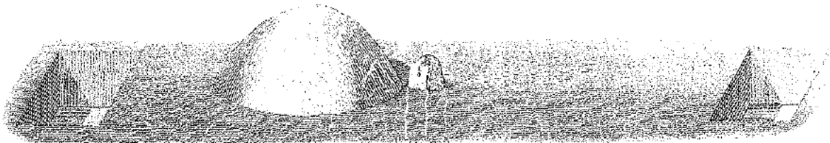
Quarter Section Corner with mound of earth
