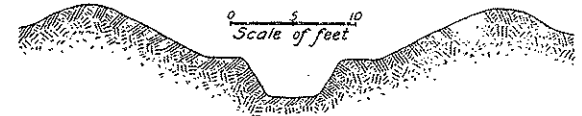
FIG. 1.—Cross section of prehistoric ditch, showing channel in bottom for carrying a small irrigating stream.
