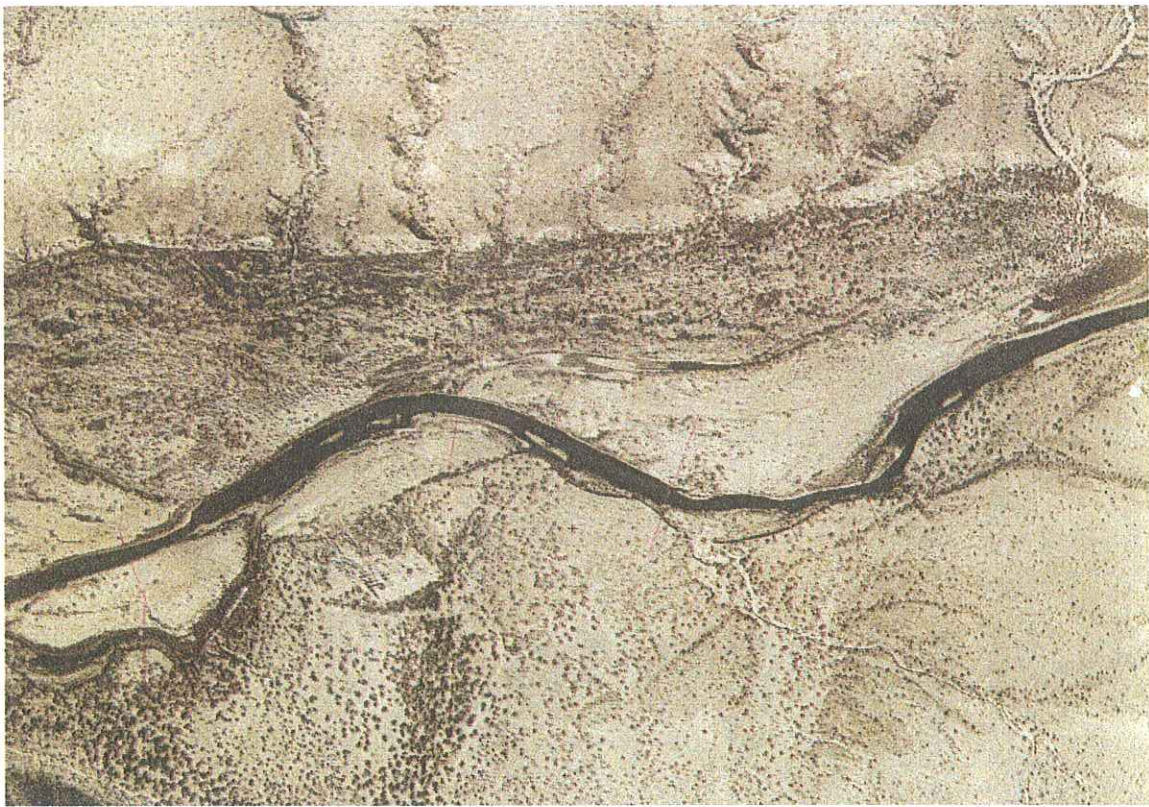
Figure 3. Braided Salt River between Blue Point and confluence with Verde River (T3N, R7E, Sec 34). Note gravel bars in low-water channel. Large areas of channel are dry and flow is controlled by upstream reservoirs.
