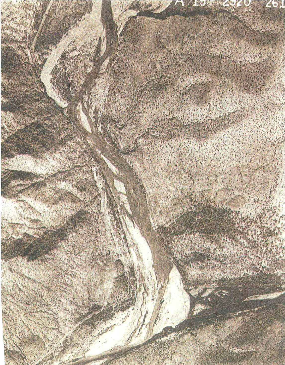
Figure 4. Verde and Salt River confluence (T2N, R7E, Sec 5). 1934 aerial photograph showing braided channel pattern and constriction. Note that large sediment delivery from Verde River forces Salt River channel to south side of valley.
