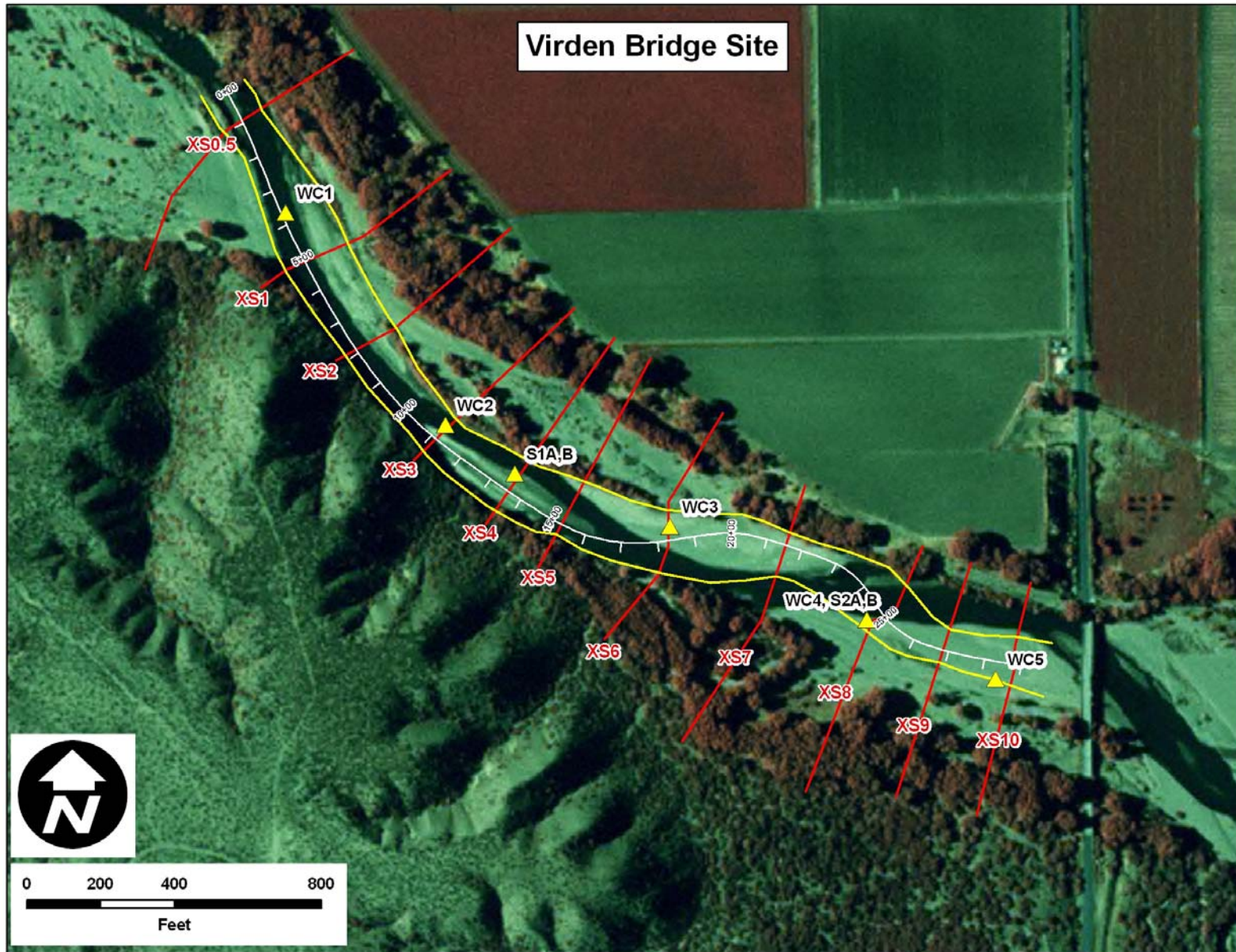
Figure 3.14. Aerial photograph showing the morphology of the Virden Bridge site, the locations of the surveyed cross sections and the locations of the sediment samples.
