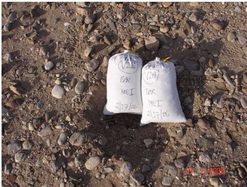
Figure A.35. Close up view of the bank-attached bar sediments (V2) at Cross Section 8 at the Virden site. The D_{50} is 4 mm and the sand content is about 33 percent.
