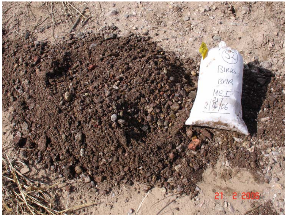
Figure A.23. Close up view of mid-channel bar sample S2 at Cross Section 3 at the Birds site. The D_{50} is 4 mm and the sand content is about 45 percent.
