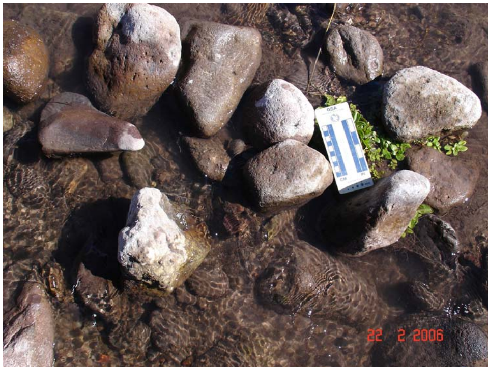
Figure A.8. Close up view of gravels and cobbles that comprise the riffle at Cross Section 4 at the Turkey Creek site at WC 2 ( D_{50} = 80 mm).
