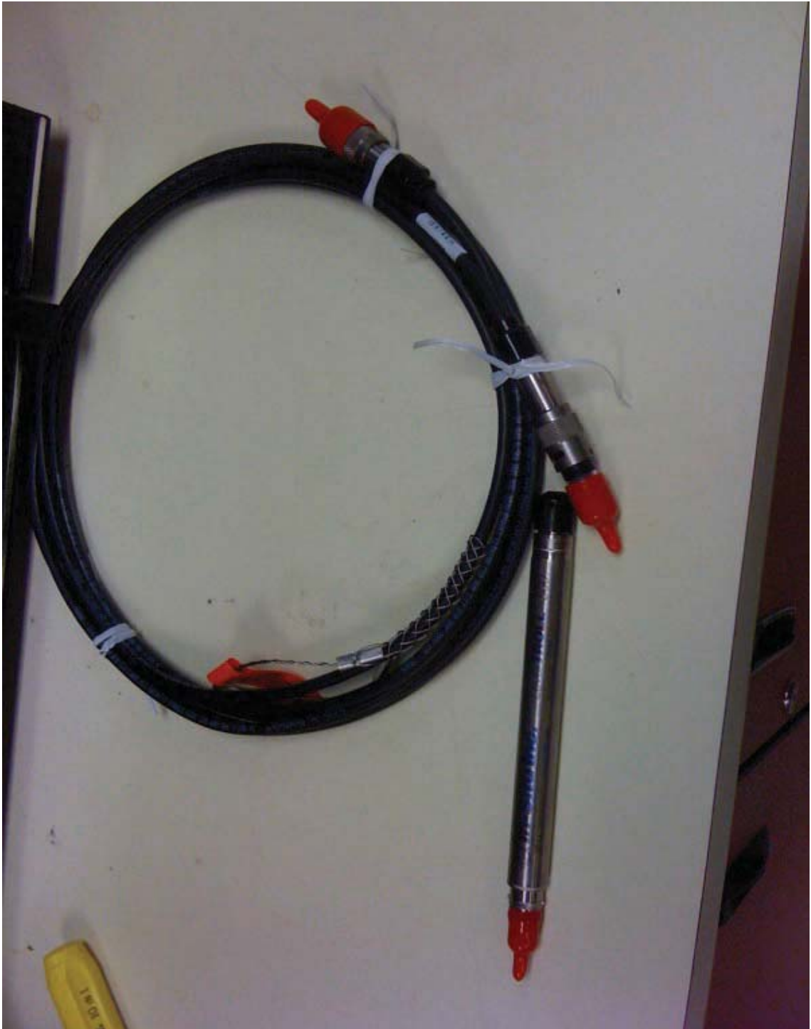
Figure 27 - Example of pressure transducers deployed at headgates and return flows of Camp Verde area irrigation ditches. Model shown is Level Troll 900, InSitu LLC, Ft. Collins, CO.
