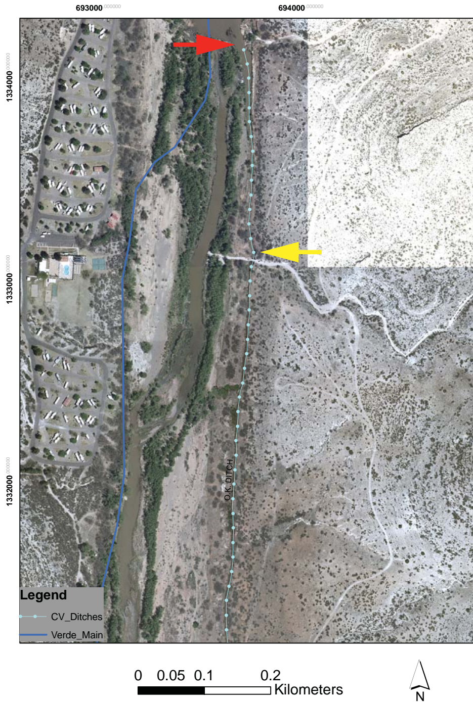
Figure 11 - Location map of OK Ditch diversion and head gates, Camp Verde, central Arizona. First major spillway of ditch is above headgate control structure. Red arrow is diversion location, and yellow arrow is head gate location.
