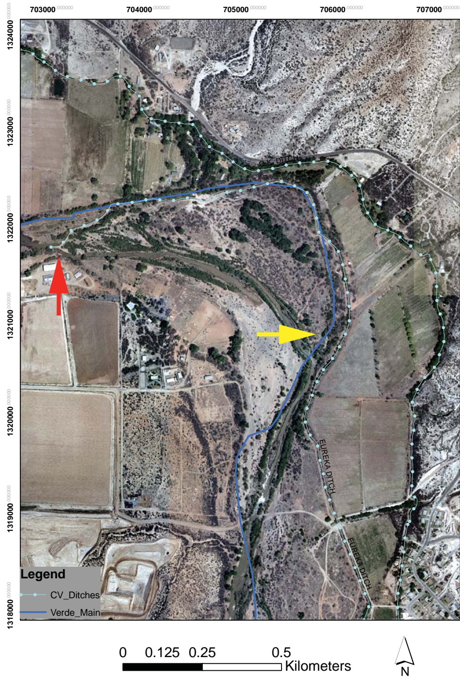
Figure 9 - Location map of Eureka Ditch diversion and head gates, Camp Verde, central Arizona. The first major spillway in on the ditch before the head gates control flow diverted into the ditch proper. Red arrow is diversion, and yellow arrow is location of head gates.
