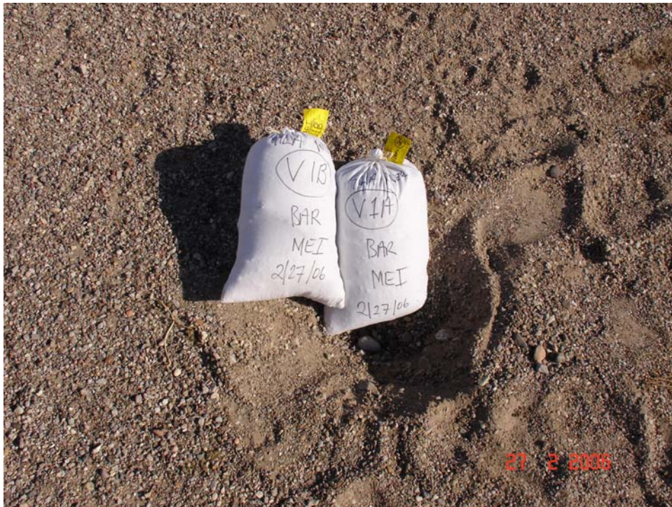
Figure A.34. Close up view of sediments deposited in the mid-channel bar at Cross Section 4 (V1) at the Virden site. The D_{50} is 1 mm and the sand content is about 55 percent.
