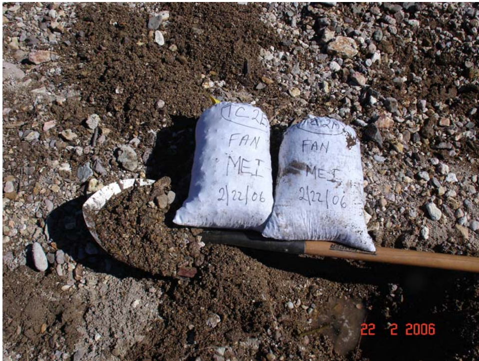
Figure A.10. Subsurface sediments on the Brock Canyon fan at the Turkey Creek site. The D_{50} is 5.2 mm and the sand content is about 35 percent.
