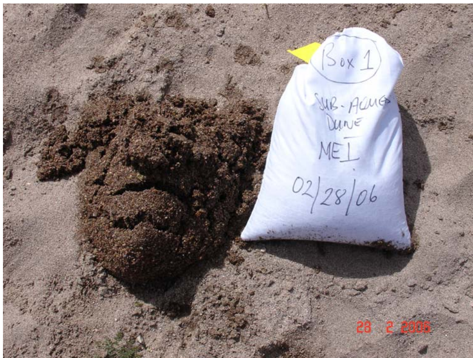
Figure A.29. Close up view of sand bed material at Cross Section 1 at the Box site. The D_{50} is 1 mm and the sand content is about 70 percent.
