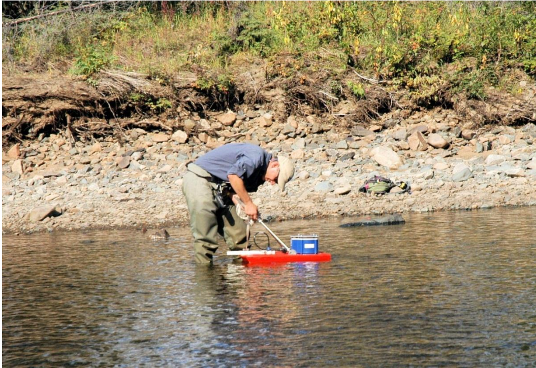
Figure 7. Discharge measurement being made at Site P7 using the StreamPro ADCP.
