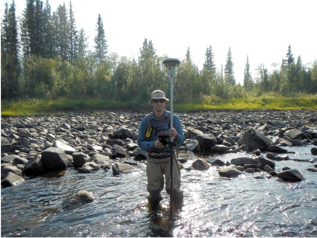
Figure 3. RTK-GPS roving unit being used by field crew to collect topographic/cross section data at Site P9. Photo by Tetra Tech field crew, August 13, 2013.
