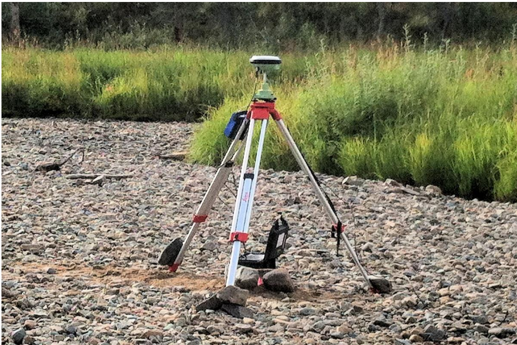
Figure 4. Typical GPS base station setup at control point for Site P3.
