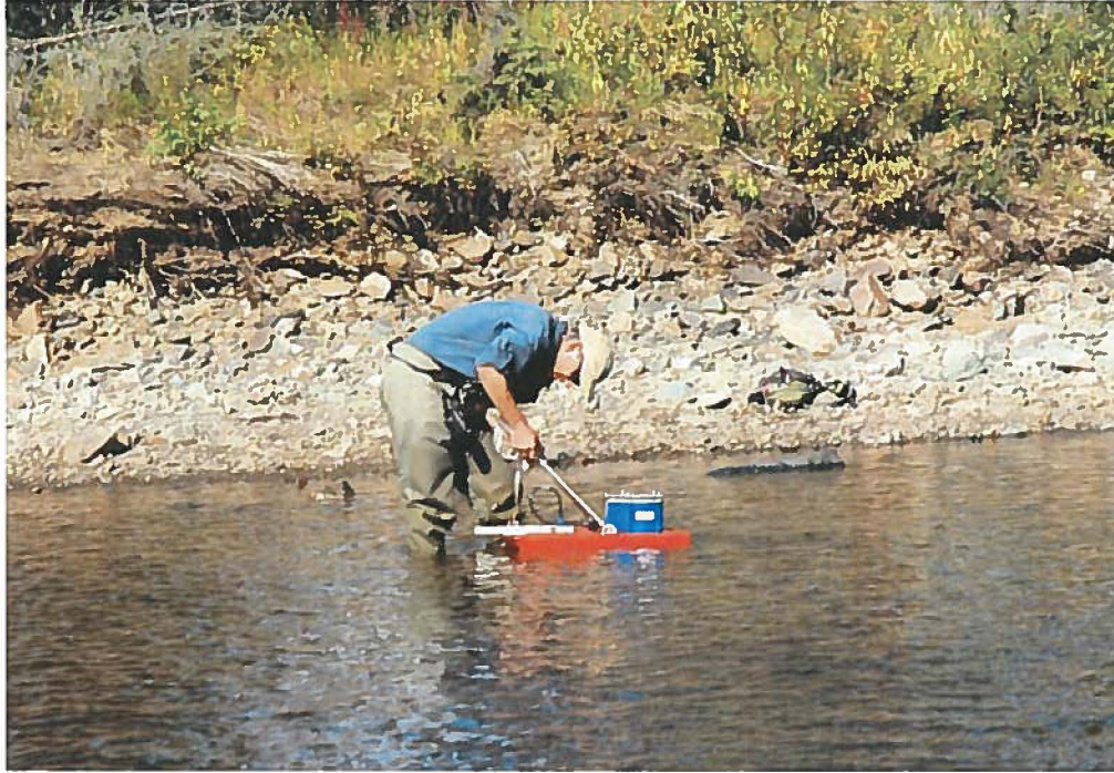
Figure 7. Discharge measurement being made at Site P7 using the StreamPro ADCP.
