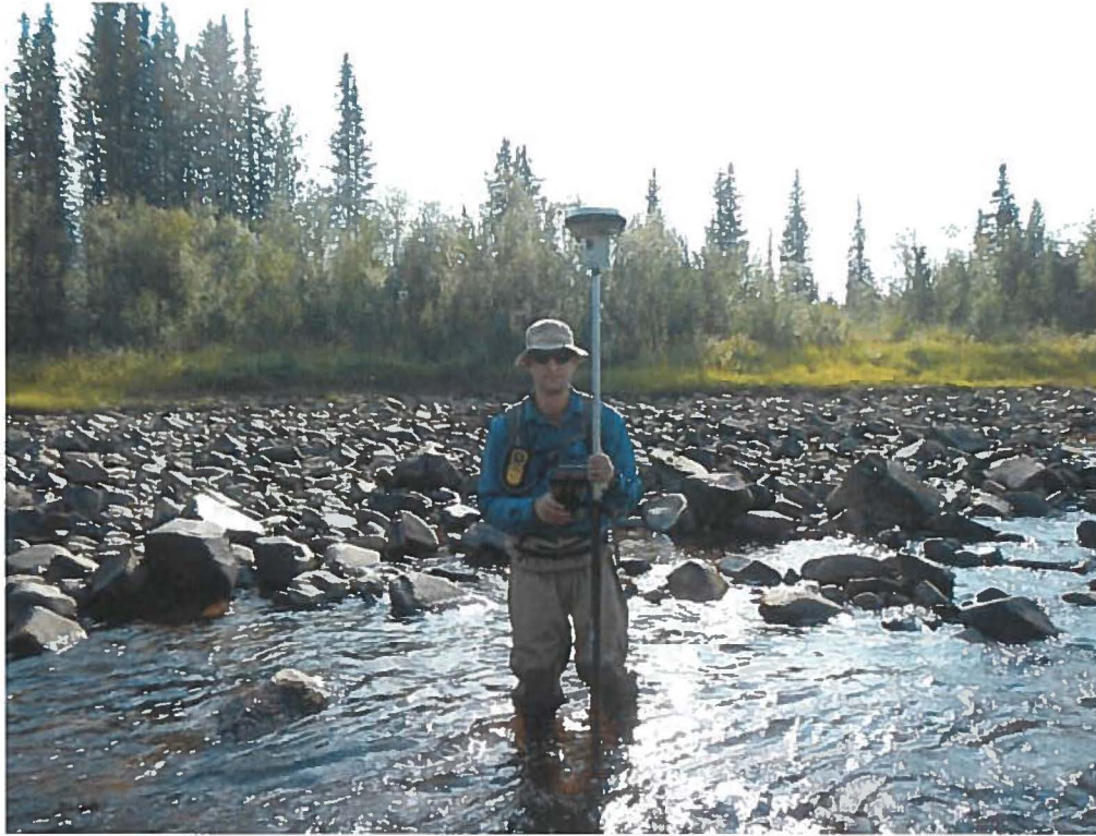
Figure 3. RTK-GPS roving unit being used by field crew to collect topographic/cross section data at Site P9. Photo by Tetra Tech field crew, August 13, 2013.
