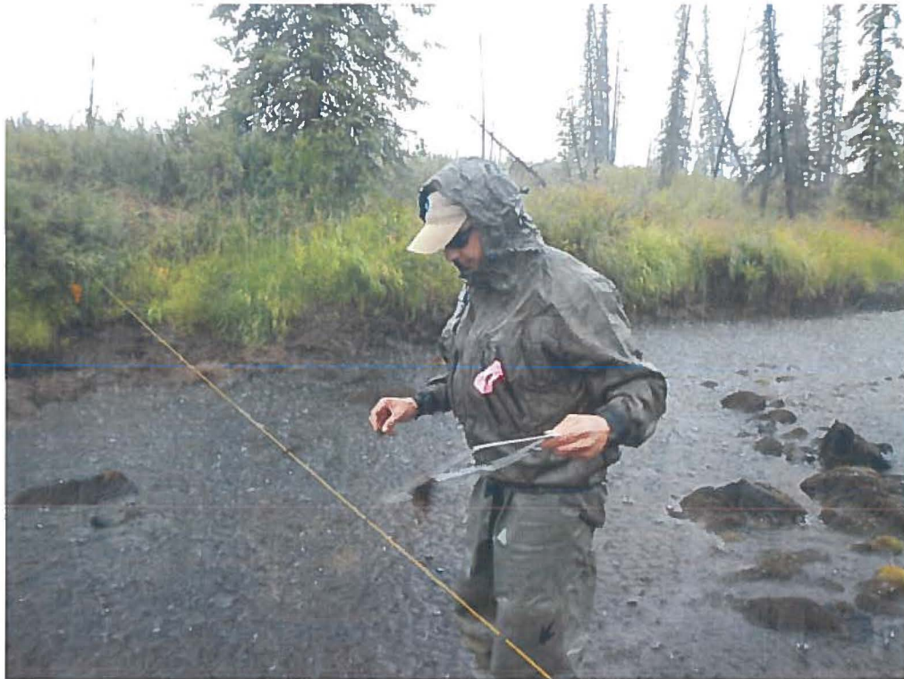
Figure 6. Sediment sample being collected using the tagline technique at the riffle near Site 1, Cross Section 5.
