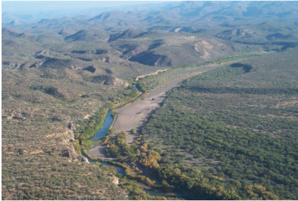
Plate 1. View upstream of Site 1 located upstream of Horseshoe Reservoir. The chute channel that extends the length of the site during flood flows is clearly visible, as is the downstream hydraulic control for the site that is formed by old alluvial fans on the right bank and a Holocene terrace on the left bank.
